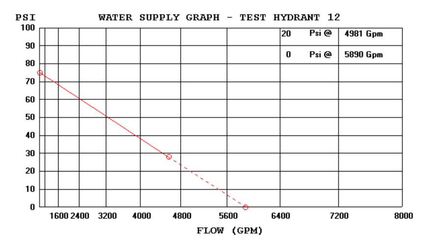
Hydrants can be classed and/or colour coded depending on the calculated fire flow at the location
